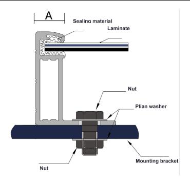
Fig. 8-1 Drawing of installation dimension
