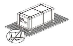
Place the unit in a dry and ventilated place.
