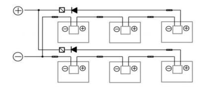
Fig. 9-3 Parallel-series Connection
