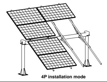
Risen module can be installed and used on the tracking system, and the installation hole position or clamp position shall be selected according to the design of the support system. Please refer to section 8.1,8.2and 8.3 for details,
