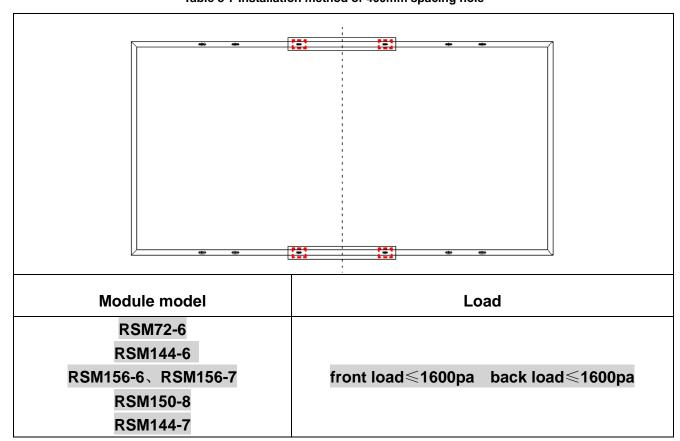
Table 8-7 Installation method of 400mm spacing hole
