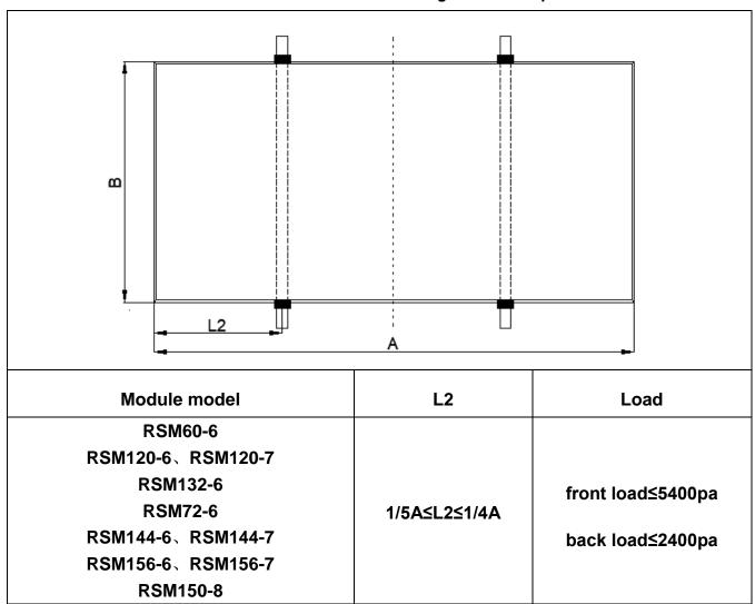
In the above installation method, the long side installation is recommended by Risen. Other installation methods unlisted above need to be confirmed with Risen professional team. System installer or trained professionals must be responsible for the design, mechanical load calculation, installation and maintenance of photovoltaic systems.
